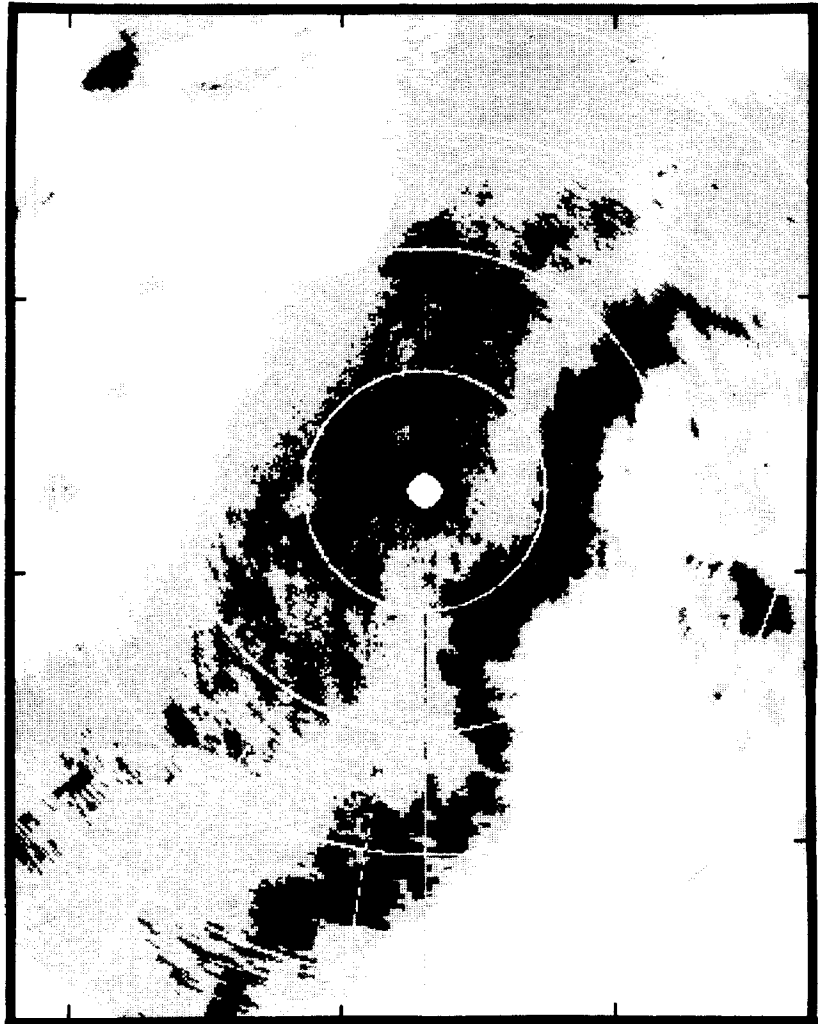
Figure 2. Low-level PPI scan of the National Weather Service Wichita WSR-57 radar at 0352 GMT 11 June 1985. Range marks are at 50 km intervals.
