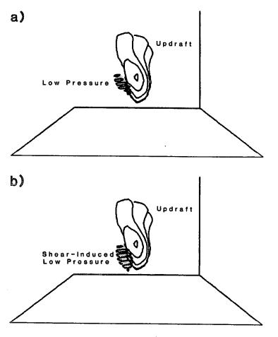
Pressure perturbations on the flank of the updraft in simulated storm with no cold pool.
