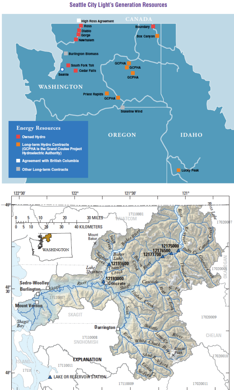
Figure 5.3. Locations of Seattle City Light energy resources. Top: Regional Map, from SCL, Integrated Resource Plan (2008). Bottom: Skagit Watershed Map, from USGS. Blue triangles represent dams: “12175000” corresponds to Ross Dam; “12176500” corresponds to Diablo Dam; “12177700” corresponds to Gorge Dam. The two other downstream dams are controlled by Puget Sound Energy as part of its Baker River Hydroelectric Project.
