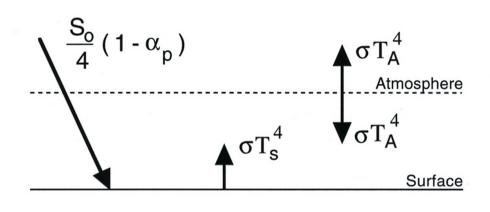
$$\frac{S_0}{4}(1-\alpha_p) = \sigma T_A^4 = \sigma T_e^4$$
