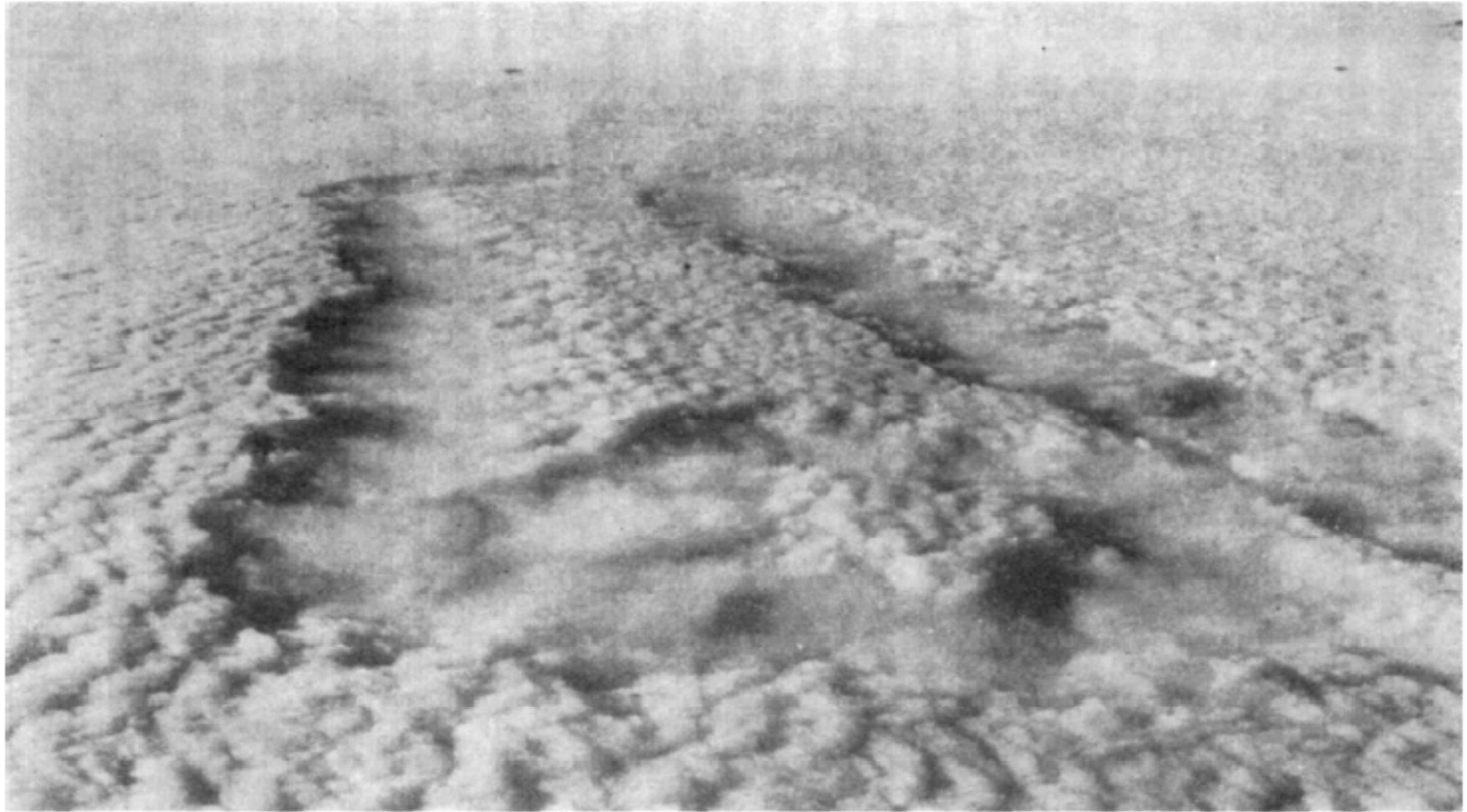
FIG. 1. The general view of the dry-ice-seeded racetrack pattern in supercooled cloud layer 37 min after the start of the seeding and 24 min after the end of the seeding. The cloud layer extended between 4500 and 6800 ft over Utica, NY, with a top temperature of -5.6^{\circ}\text{C} . The picture was taken at 1521 UTC 24 Nov 1948 from an altitude of 17 630 ft. (From Langmuir 1961b.)
